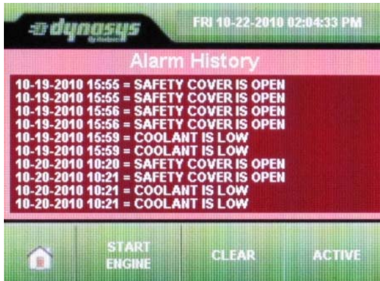
Figure 8 Alarm History Screen
