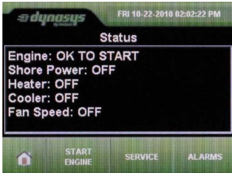
Figure 5 Engine Status Screen
